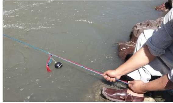
Sonar attached to graduated rope
