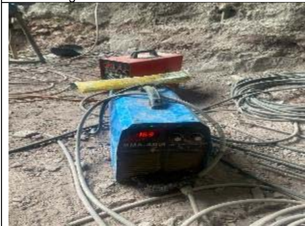
The thimbles of the welding machine observed damaged
